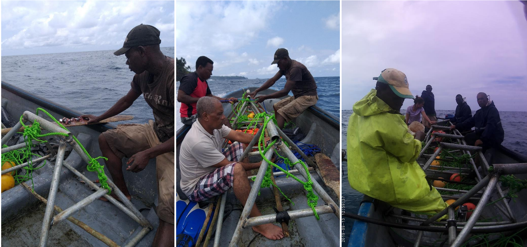
Figure 5: Marine team in São Tomé: A) Bait was chopped on the paddle before putting it in the bait cages; B) Preparing the BRUV devices for their deployment included: attaching the ropes with the buoys and the poles bearing the bait cages to the devices; C) Five BRUV devices ready to be deployed. All pictures by Guillermo Porriños.
