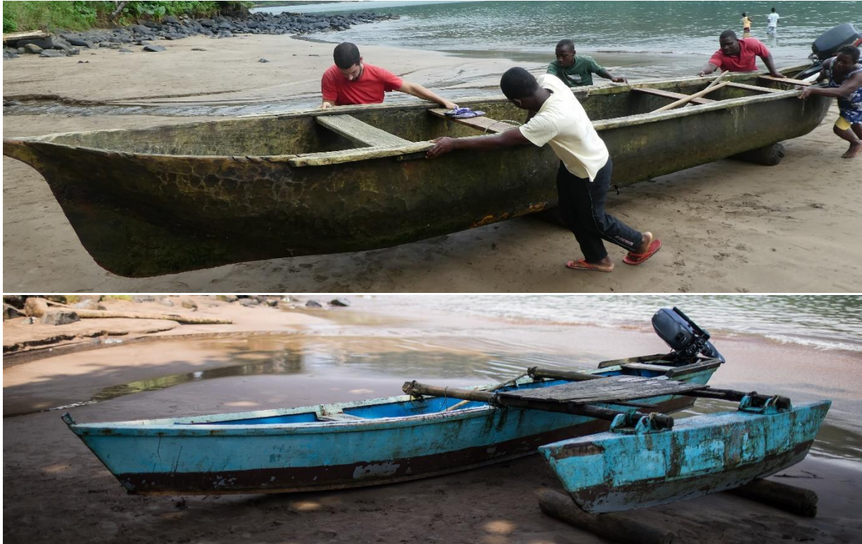
Figure 2: Main types of artisanal fishing boats used in São Tomé and Príncipe. A) Engine-propelled dugout canoe being pulled out of the water in Hospital Velho (Príncipe Island) (© Gisela Costa); B) “Prao” outrigger (Hospital Velho, © Dário Pequeno Paraíso)
